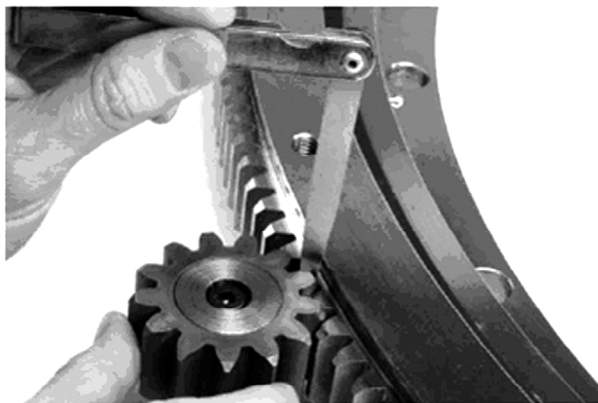
Picture 3-3 lateral clearance inspection
